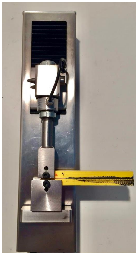
Figure 13. DCB test setup.
