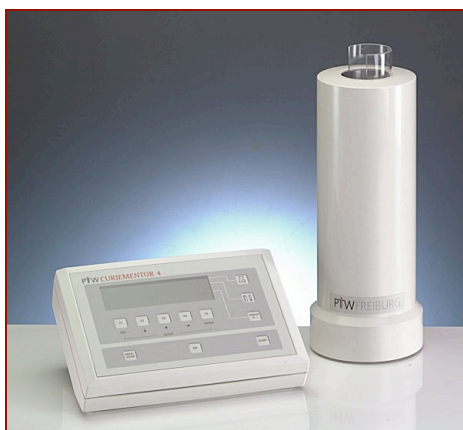
Figura 19. Curiementor 3 Isotope Calibrator
