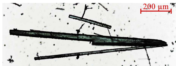
Figure S6.1: Optical Microscope image of TCP-MOF1 crystals.
