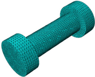
Figure 62. Model parts mesh, refined in the most critical areas
