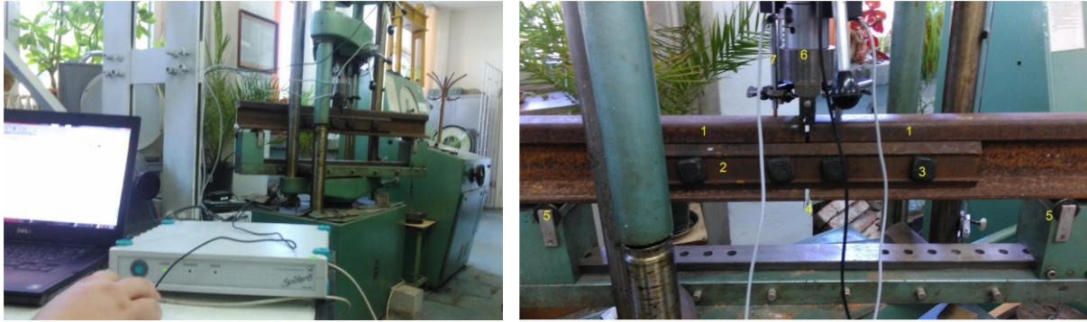
Figure 33. Laboratory three point bending test on IRJ [27]
