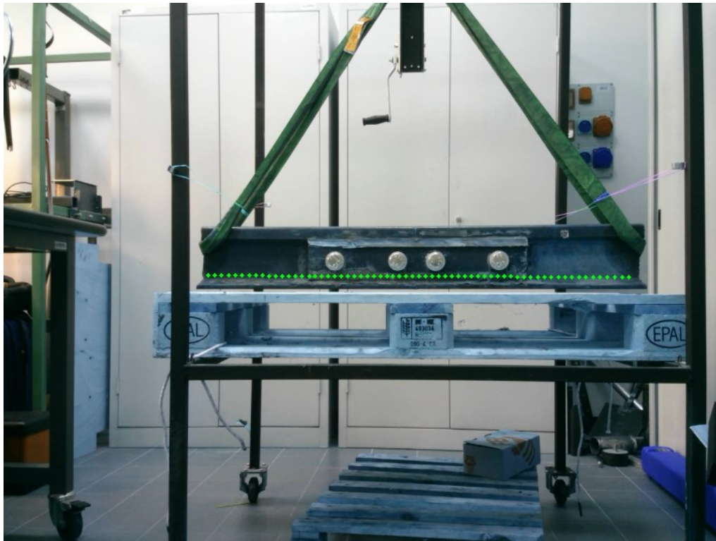
Figure 96. IRJ region scanned by LiDAR
