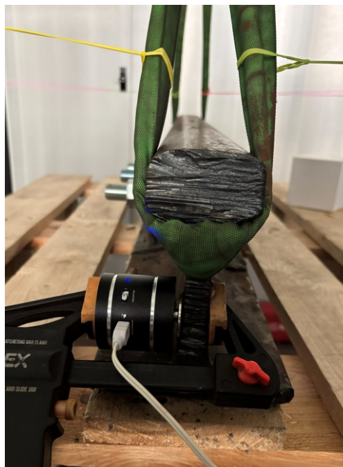
Figure 35. IRJ excited by shaker
