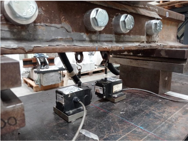
Figure 76. Linear potentiometric displacement transducers set up
