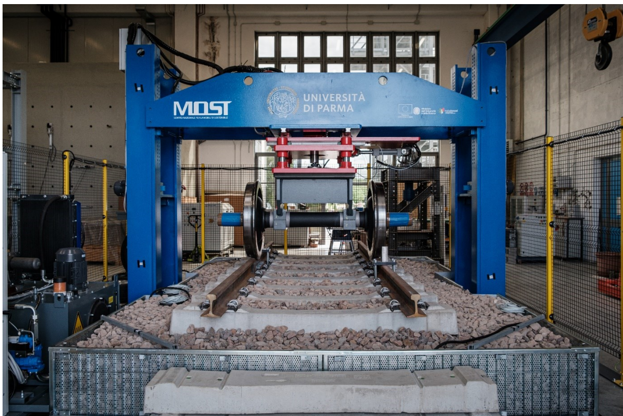
Figure 105. Railway superstructure full-scale prototype
