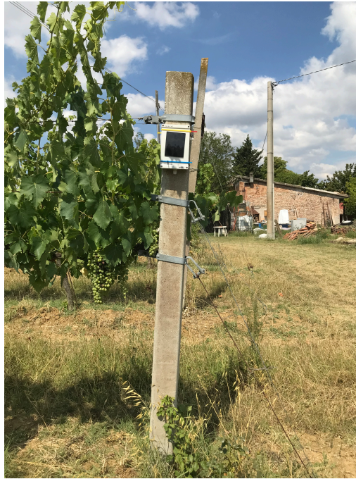
Figure 3.16: An EN (SN-V1) belonging to the vineyard module deployed in the Podere Campáz.
