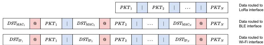
Figure 2.3: Data packets format of the proposed MIG to exchange data with end targets.
