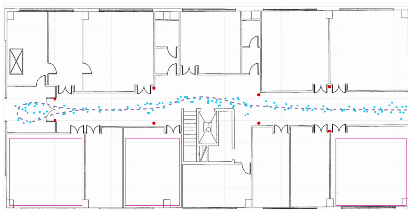
Figure 5.3: Experimental results of the UWB localization application on a sub-250 gr quad-copter. Red dots: represent the anchors positions; cyan dots: represent the estimated real-time position of the UAV; purple dashed line: is the ground truth trajectory followed by the UAV during the experimental flight.
