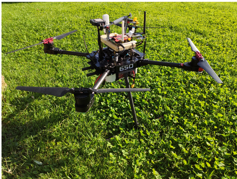
Figure 2.22: Aerial MIG located on the Tarot 650 quad-copter.
