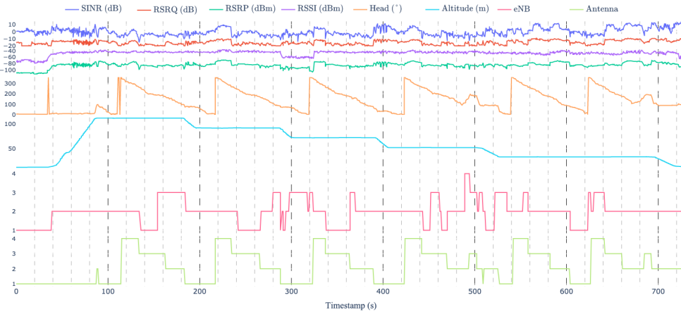
Figure 4.13: Directional antennas with NBTS algorithm LTE radio signal behaviour along the pre-defined flight path.
