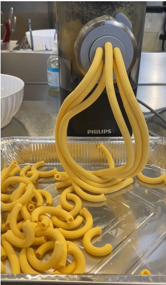
Fig. 2. Extrusion phase with the extruder machine equipped with a die for maccheroni.
