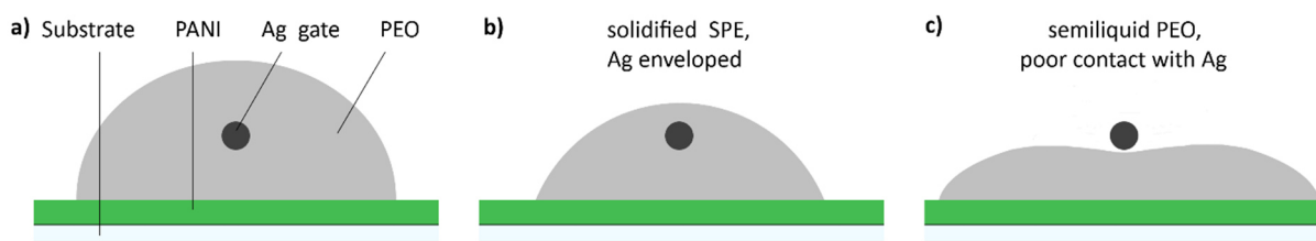
Figure 4-32: Schematic representation of the deposition of a PEO gel in the active zone of an OMD a), followed by an ordinary drying process with the gate electrode staying emerged in the SPE (b). c) Supposed drying process of gels with excessive dopant hygroscopicity and/or chaotropicity (such as P30-AB-05, P30-AB-10), leading to insufficiently contact of the gate electrode with the electrolyte.
