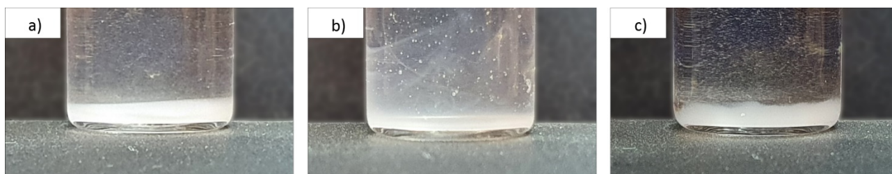
Figure 4-25: Precipitate on the bottom of a vial containing a one-month-old, 30 mg/ml PEO gel sample made with 0.1 M \text{AlCl}_3 and 0.05 M \text{LiClO}_4 a) prior to agitation, b) immediately after, c) 30 min after agitation. The dots that can be seen in the bulk of the gel after agitation are air bubbles.
