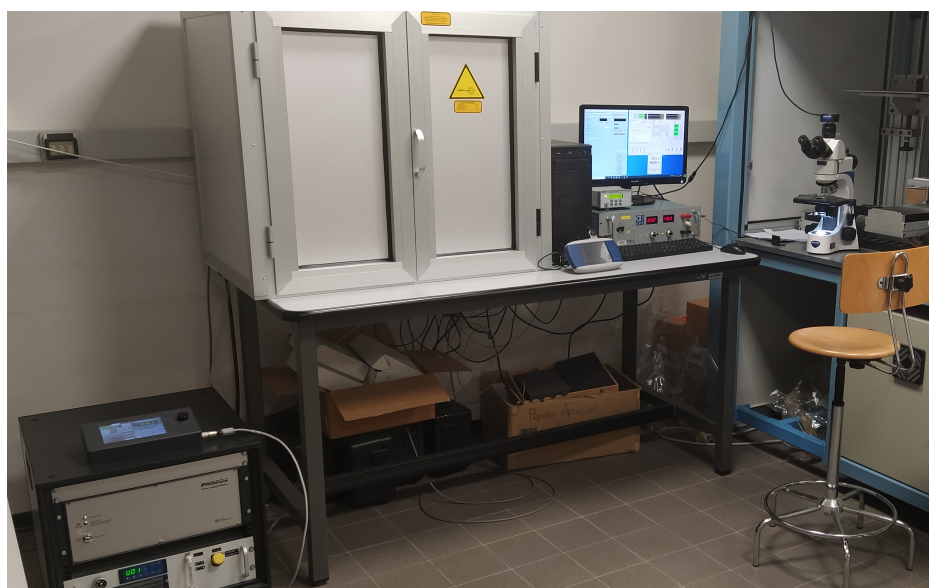
Figure 3.2: A photograph of the laser source and instruments employed for microfabrication via TPP.
