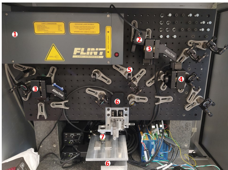
Figure 3.3: Photograph of custom-built TPP setup.
