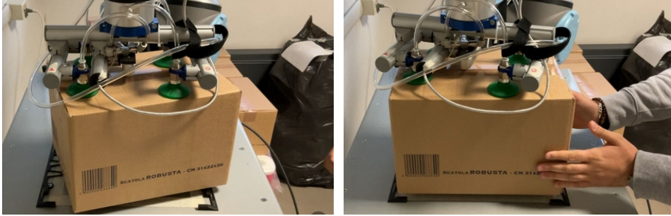
Figure 4.7: Placement of a cardboard box above the deposit fixture \mathcal{D} without displacement error correction (left) where it can be observed that the gripper is aligned to the deposit fixture, while the box is not. Placement of a cardboard box inside the deposit fixture \mathcal{D} with manual error correction (right image) to compute the ground truth error correction.
