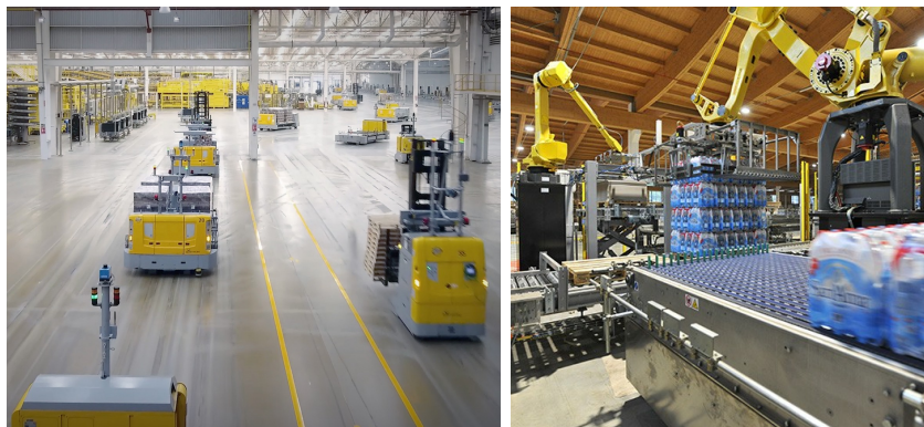
Figure 2: Example of AGVs and LGVs fleet produced by E80 Group S.p.A. (left) and fixed manipulation stations (right).
