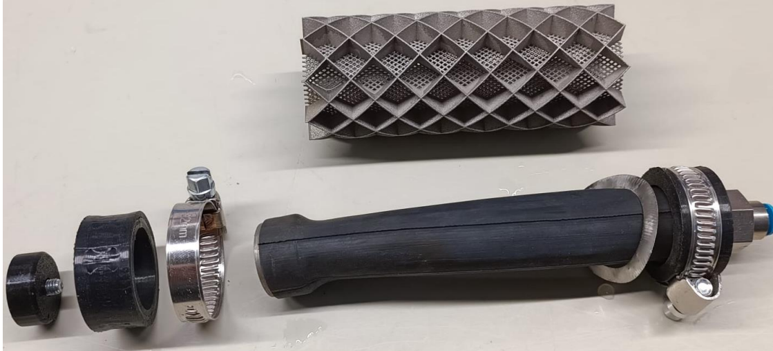
Figure 4.7 Setup of the tube carrying out pressure and the sealing components.
