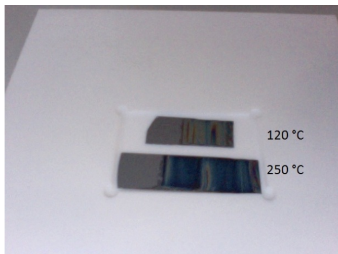
Figure 1.2.1. Example of film formed on silicon wafers after heating at 120°C and 250°C before rinsing with distilled water
