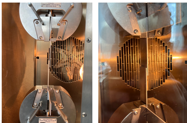
Figure 6.11. Pictures of lap shear test performed at 180°C. In the left picture is visible the two aluminum joints already detached before the measurements, on the right the sliding of the specimen.
