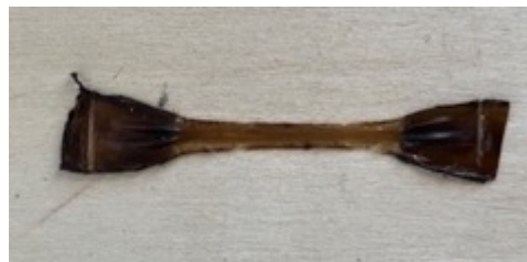
Figure 3.22. Appearance of LCE-9%QxCav u after alignment process.
