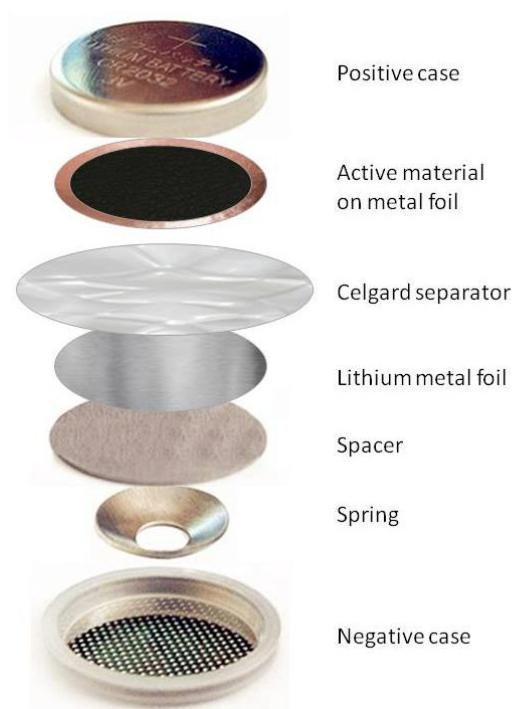
Figure 4-4 CR2032 coin cell. This schematic representation shows the standard architecture of any electrochemical device produced and investigated in this thesis work. Titania and sulfur battery employ aluminum foils as collectors. The system is soaked in suitable electrolyte.
