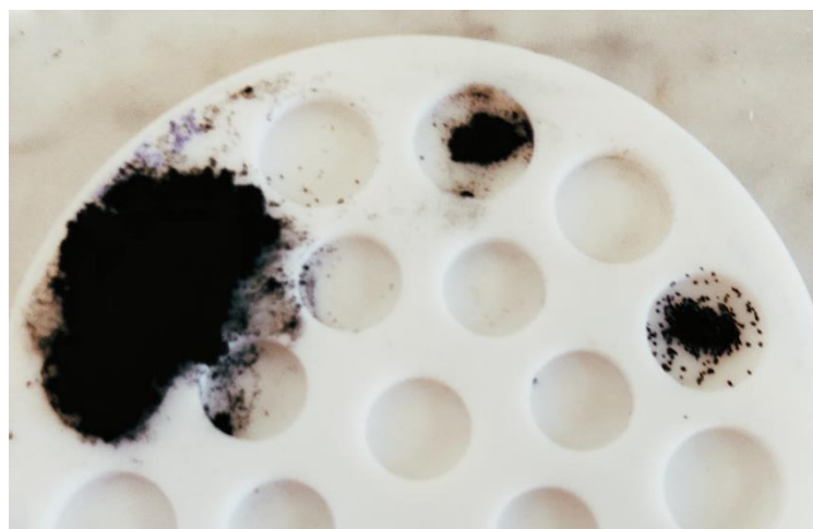
Figure 5-26 Different appearance of sulfur-carbon composites. From left to right, clockwise: S - TEGO dT, S - TEGO BM and S - LAArGO.
