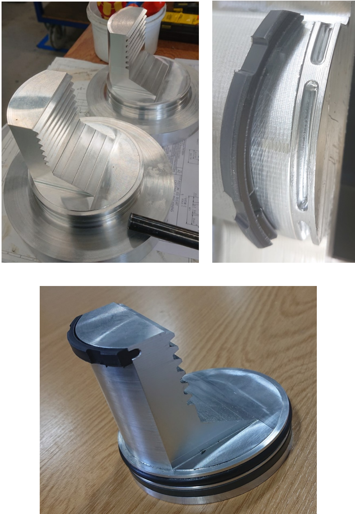
Figure 70. Piston prototype obtained by machining to be used for the validation of the new sliding pads design.
