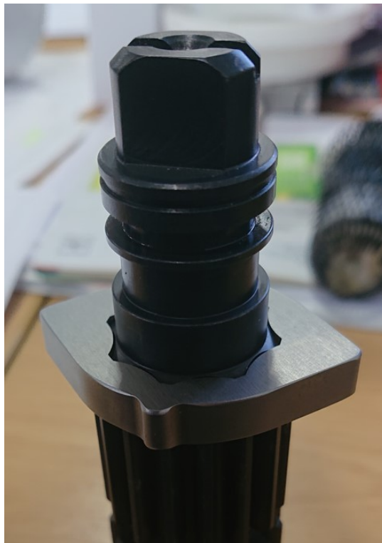
Figure 71. Preparation of the prototypes of cam, stud bolts and pinion for the validation of the new angular stroke adjustment mechanism via actuator mockup prototype.
