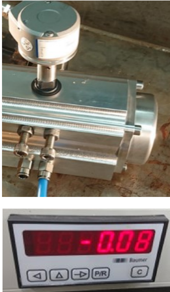
Figure 64. Validation test of the cam system with angular deformations measurement. A digital angle sensor provided with a digital display is connected to the pinion.
