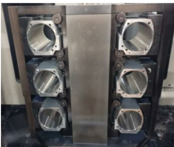
Figure 36. Positioning of center bodies on jigs for machining with CNC machines.
