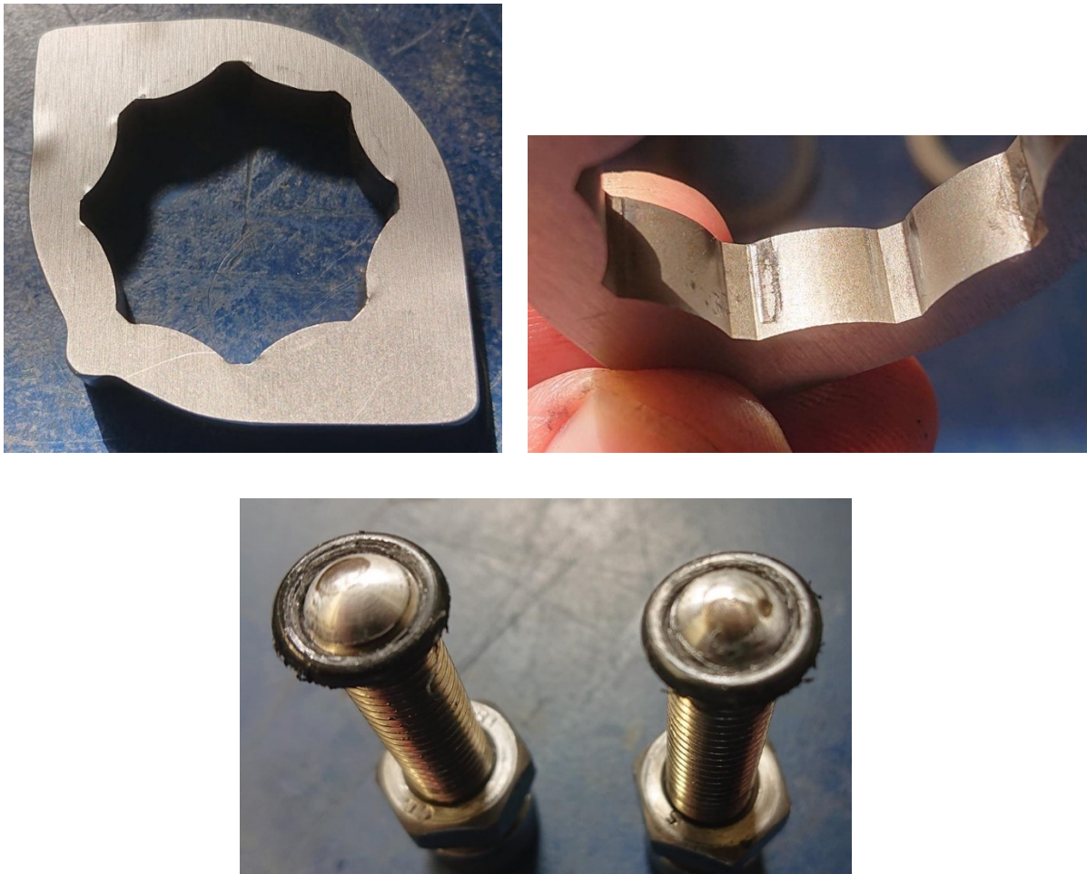
Figure 69. Check of the components of the cam - stud bolts connection after high pressure cyclic test.
