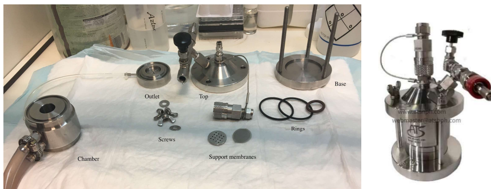
Figure 2.45: Components of extruder (left) and their assembly (right).
