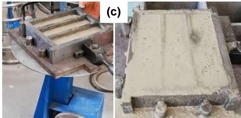
Figure 1. Preparation of GO-B specimens: (a) fresh slurry, (b) flow table test, (c) fresh slurry compacted in prismatic moulds.
