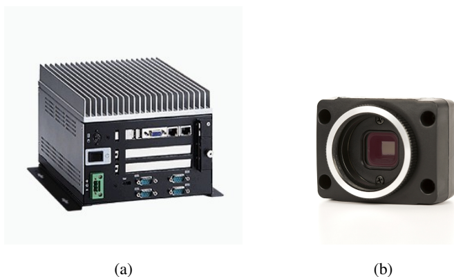
Figura 3.4: PC Industriale Axiom IPC910H a ed telecamera Modello FireFly MV b .
