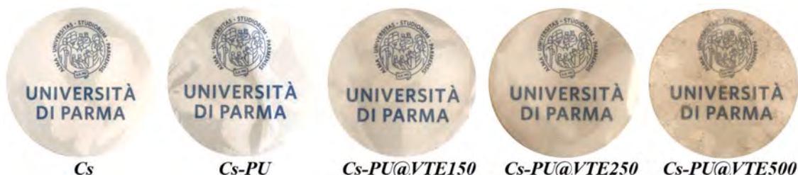
Fig. 6. Physical appearance of Cs, Cs-PU and Cs-PU@VTE films.
