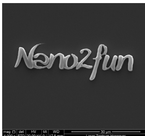
Figure 1.7: SEM image of Nano2Fun logo fabricated via two-photon polymerization in Laser Zentrum Hannover (LZH) during the 5th meeting of ITN Nano2Fun.
