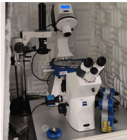
Figure 2.33: picture of the setup used for the nanomechanical measurements. It is placed on an active vibration isolation optical table as well as in an acoustic enclosure.
