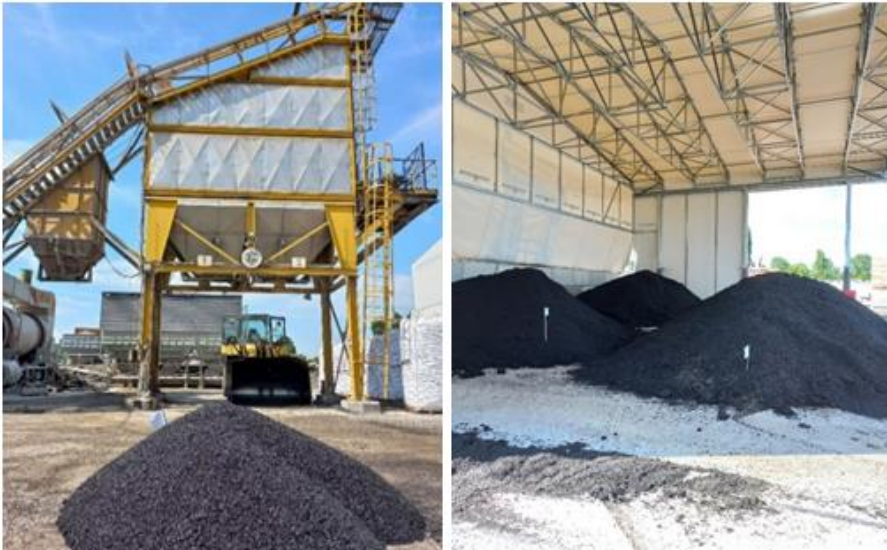
Figure 5.1. CMPM production, discharge, and storage
