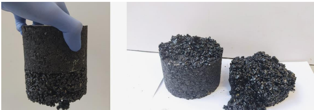
Figure 1.9. Adhesion test on the inverted complex specimen
