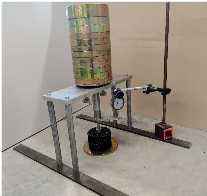
Figure 3.3. Indentation test device
