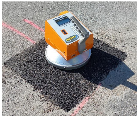
Figure 6.8 Measuring the densities of patches with a non-nuclear electromagnetic density gauge
