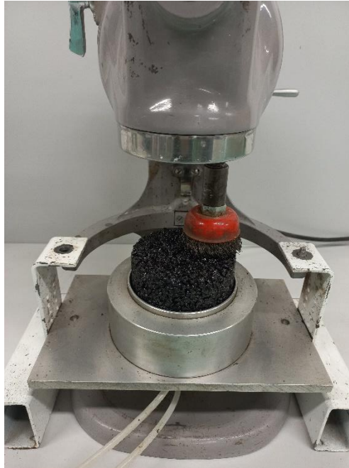
Figure 2.9. Conducting the brush test to assess the raveling of CMPMs
