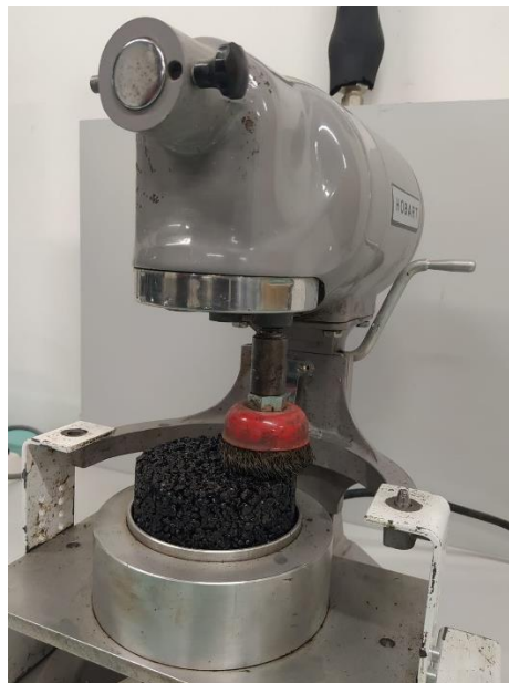
Figure 3.4. Conducting the brush test to assess the raveling of CMPMs
