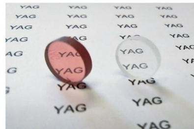
Fig. 4. Photograph of YAG ceramics containing Si (0.5 wt% TEOS) and a small amount of Zr (introduced by milling process) sintered in vacuum at 1735 °C; after vacuum sintering, the sample has a red coloration (left), which disappears after annealing in air (right). (For interpretation of the references to color in this figure legend, the reader is referred to the Web version of this article.)
