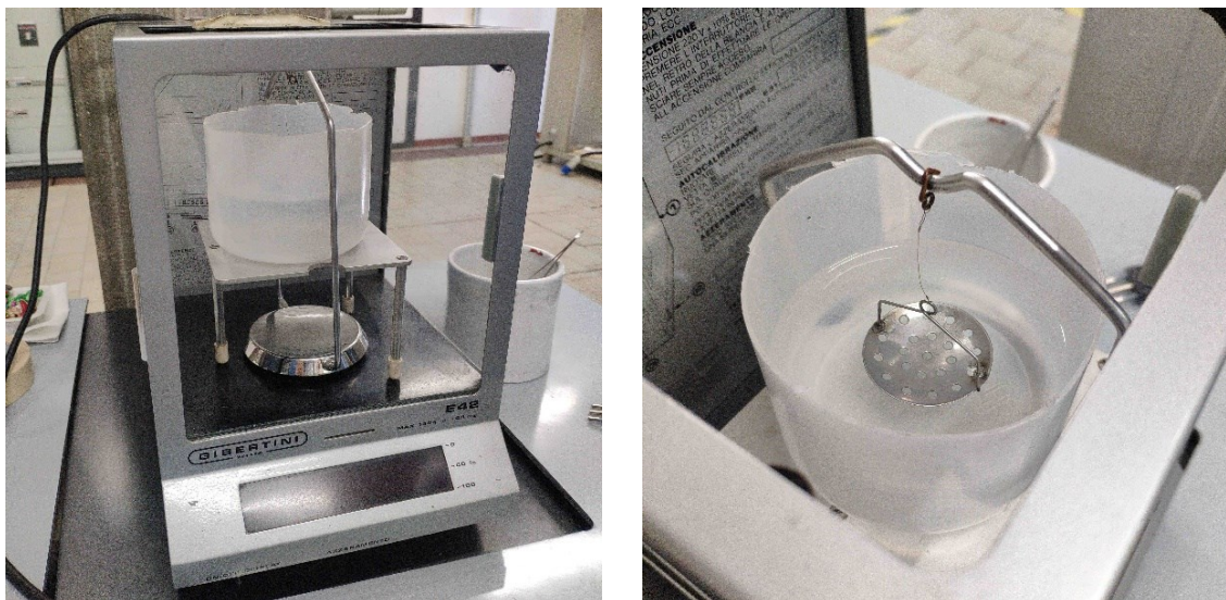
Figure 2-1 Scale used to measure the density by Archimedes' method.
