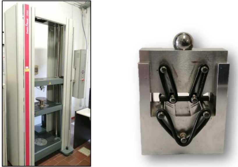
Figure 3.13 Illustration of Z050, Zwick-Roell (left) and a semi-articulated test fixture for the four-point bending strength test (right).
