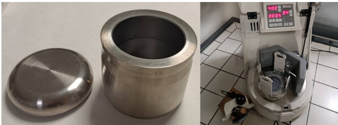
Fig. 3.1 WC jar and planetary mill (Pulverisette 6 Classi Line, Fritsch Planetary Mill).
