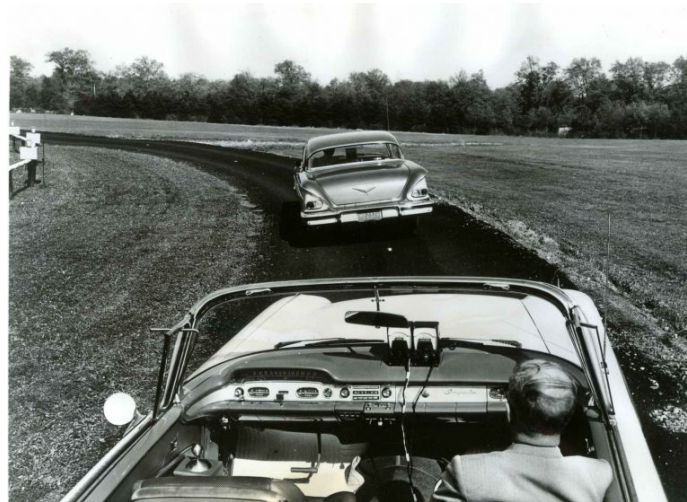
Figure 4: Test on the driverless car developed by RCA Labs , which used sensors to detect an electrical cable embedded in the road carrying warning signals
