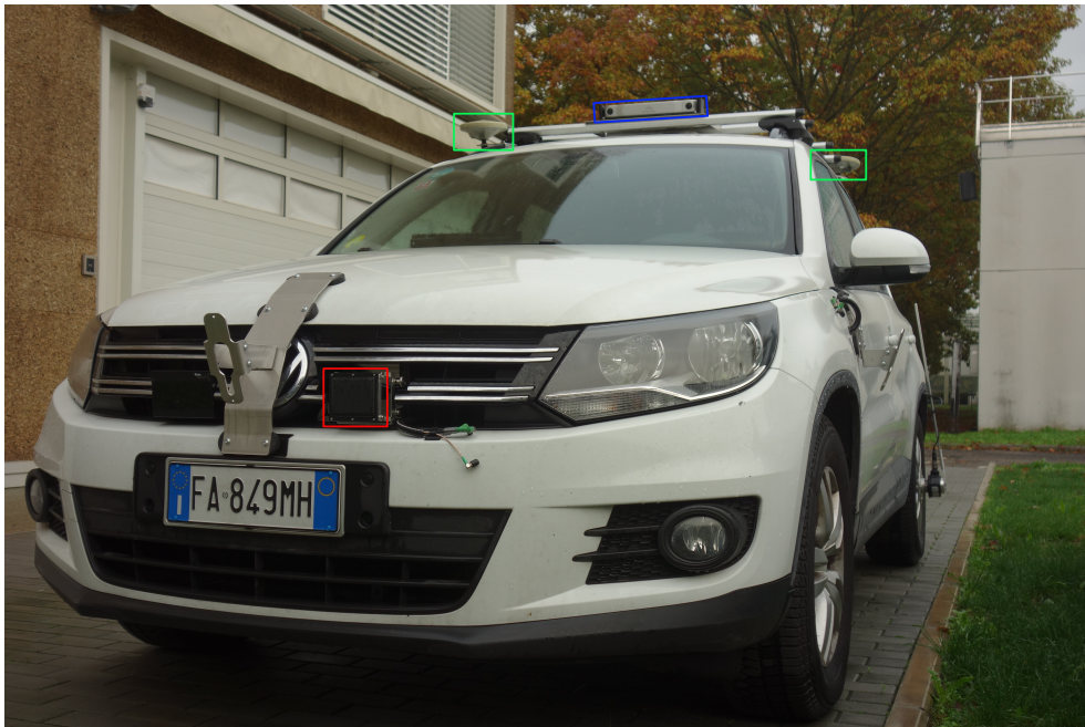
Figure 4.6: Volkswagen Tiguan used as test vehicle for acquiring real-world data; in red it is highlighted the radar used for detecting obstacles, in blue the camera for recording images and in green the antennas of the GNSS-INS positioning system
