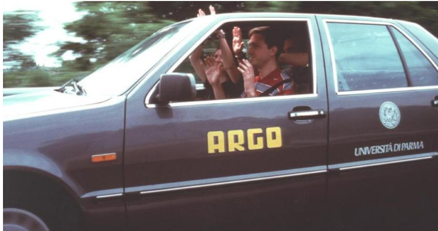
Figure 7: Argo, the autonomous Lancia Thema developed at the University of Parma
