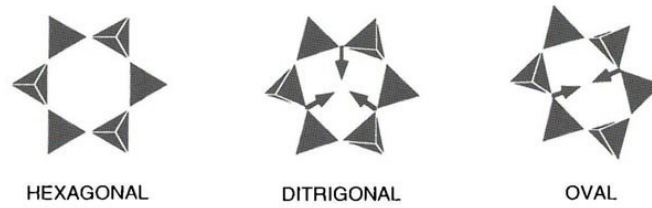
Figure 8 – Two possible distortions of the hexagonal ring as a result of the rotation of the \text{SiO}_4 tetrahedra [36].
