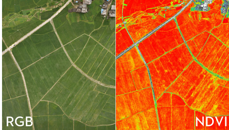
Figure 1: Example an RGB image (left) and derived NDVI index (right), illustrating how multispectral data can quantify vegetation health. Green color indicates a good vegetation health, while red color suggests bad vegetation health. [1]
