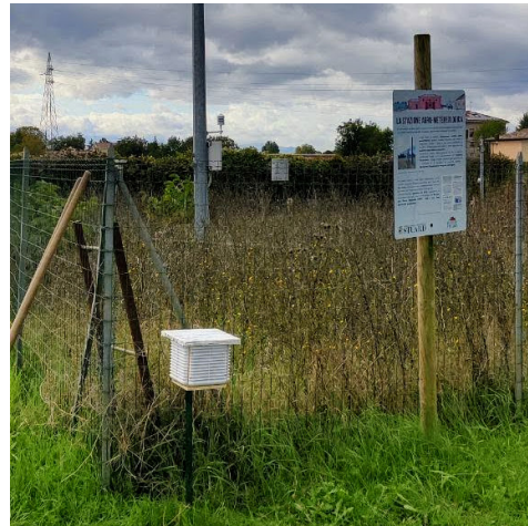
(b) Deployment in field of the air-permeable, waterproof data collection node near the ARPAE "San Pancrazio" weather station in Parma, Italy.
