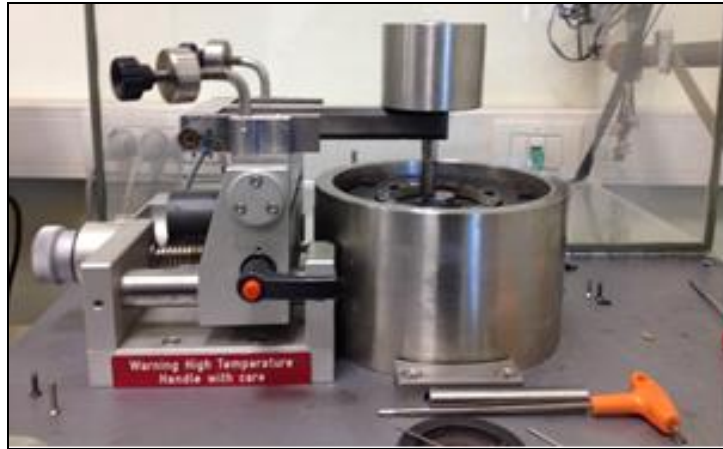
Figure 1.13: CSEM High Temperature Tribometer.
