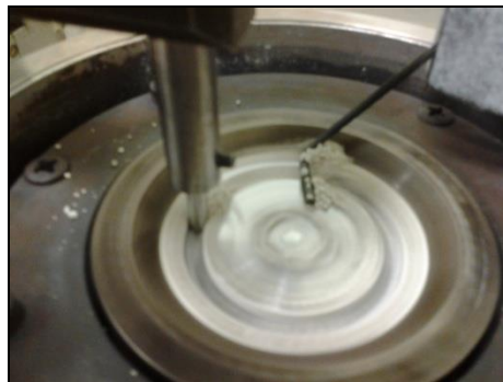
Figure 1.14: “powder test” configuration
