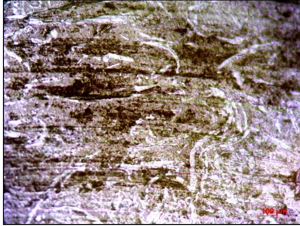
Figure 3.7: Optical microscope image in bright field of tribological trace.
