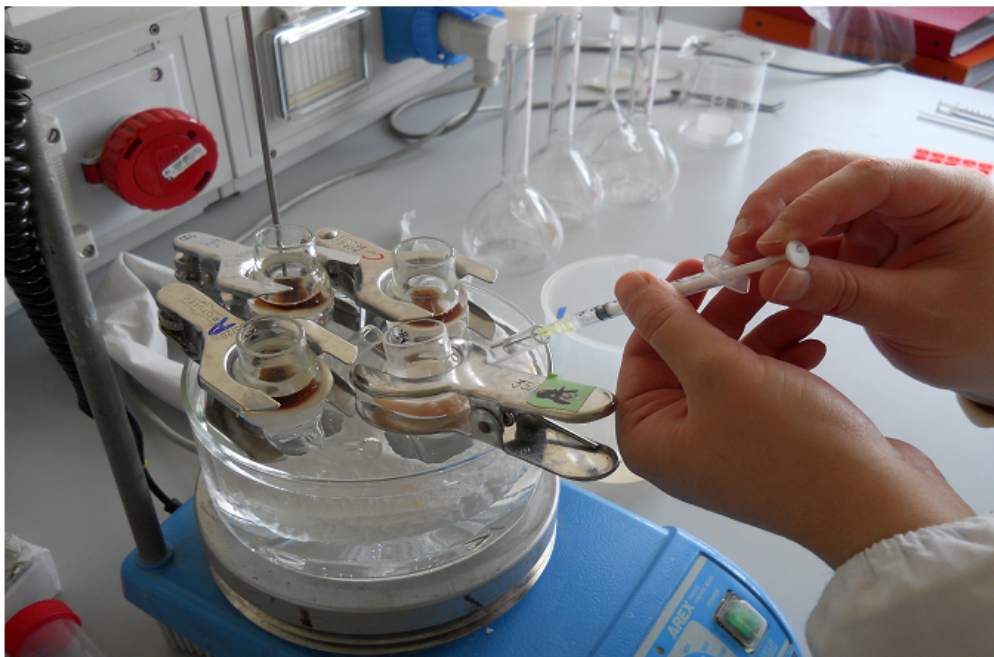
Figure 10. Setting for permeation test
