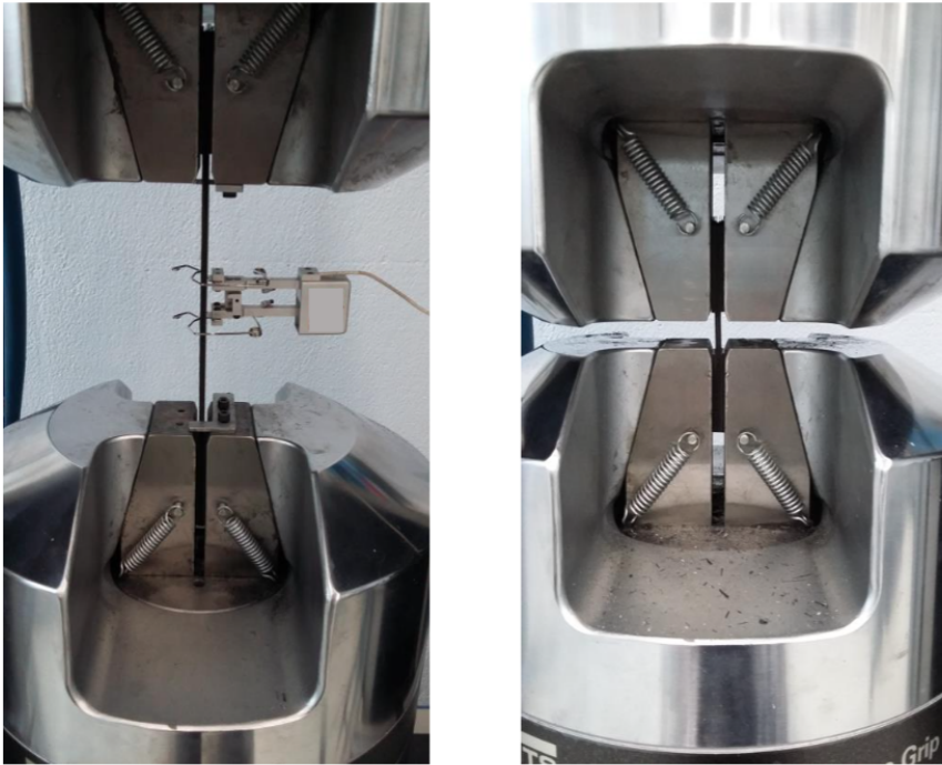
Figure A.4: MTS Insight electromechanical testing system used for uniaxial tensile (left) and compressive deformation testing (right).
