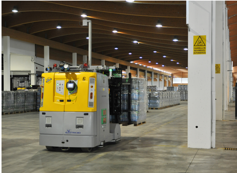
Figure 3.1: An industrial Ackermann AGV with visible front steering and actuated wheels, its back forklift and a navigation laser scanner at the top of a telescopic pole. Although with slightly different mechanical structure, Dual Drive AGVs have a similar appearance.
