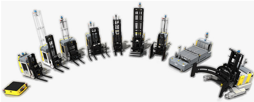
Figure 1.1: Different Autonomous Guided Vehicles (AGVs) manufactured by Elettric80 SpA with different material movement tools installed (forks, pantographs, conveyors or clamps).
