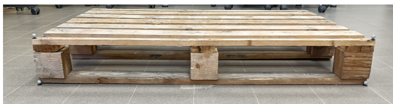
Figure 4.8: OptiTrack marker placed on the pallet.
