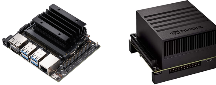
Figure 2.7: Jetson Nvidia production. On the left the Nvidia Jetson Nano, on the right the Nvidia Jetson AGX
