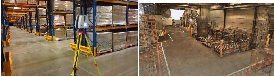
Figure 2.1: On the left, a terrestrial laser scanner on a tripod acquiring 3D scan of the warehouse. On the right, an example of 3D point cloud acquired.
