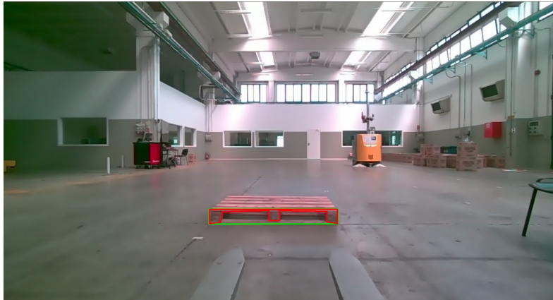
Figure 4.13: Example of detection. The green rectangle is the bounding box. The red lines connect the keypoints.
