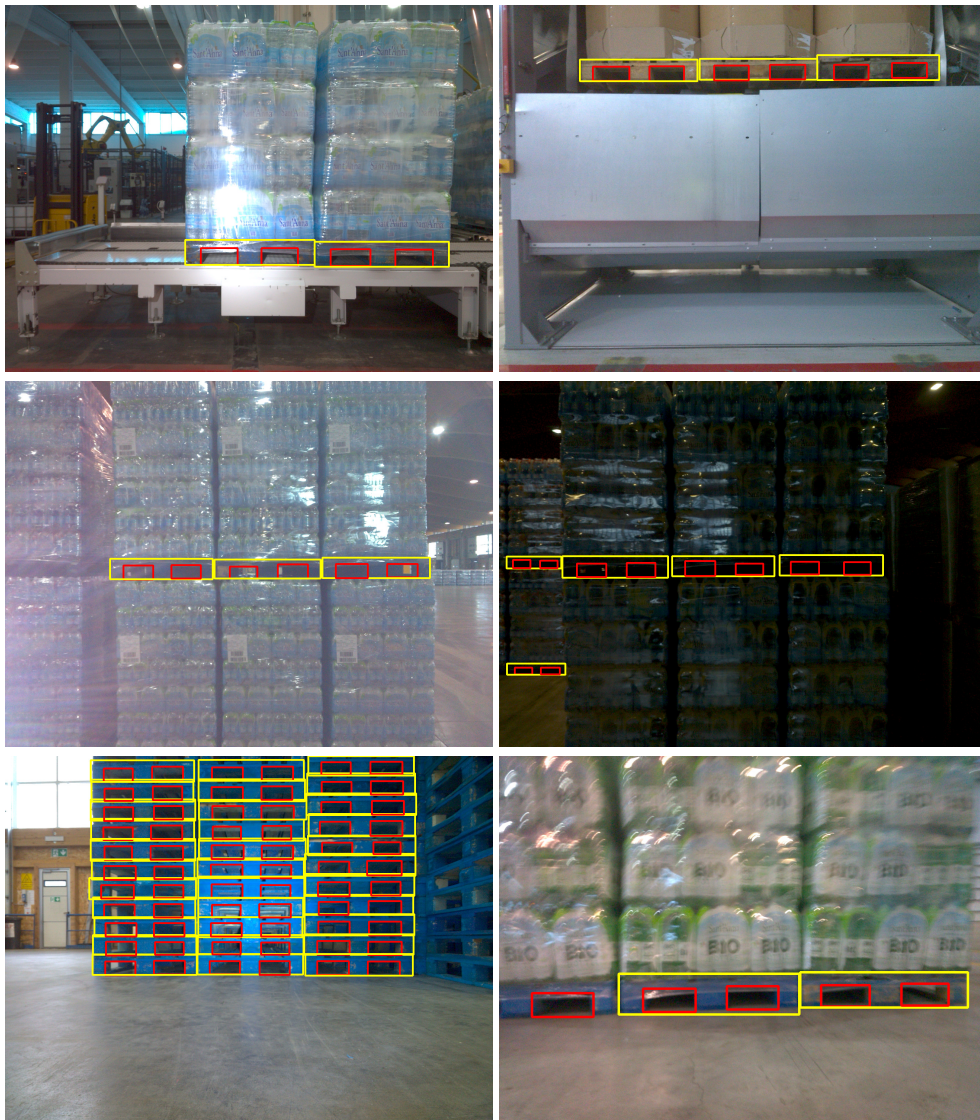
Figure 3.6: Examples of detected front sides of pallets and pallet pockets using Faster R-CNN.
