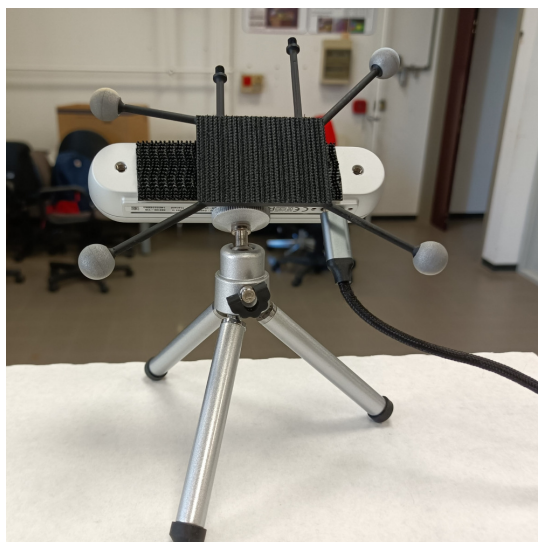
Figure 4.6: Rigid body markers on the back of the camera case.
