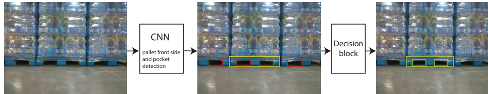
Figure 3.1: Proposed pipeline for automatic pallet detection (from left to right). Each input RGB image (left image) is first processed by a CNN (center image) to detect the front sides of pallets (yellow boxes) and the pallet pockets (red boxes). Then, a decision block is applied to select the final pallet proposals (right image, green color).
