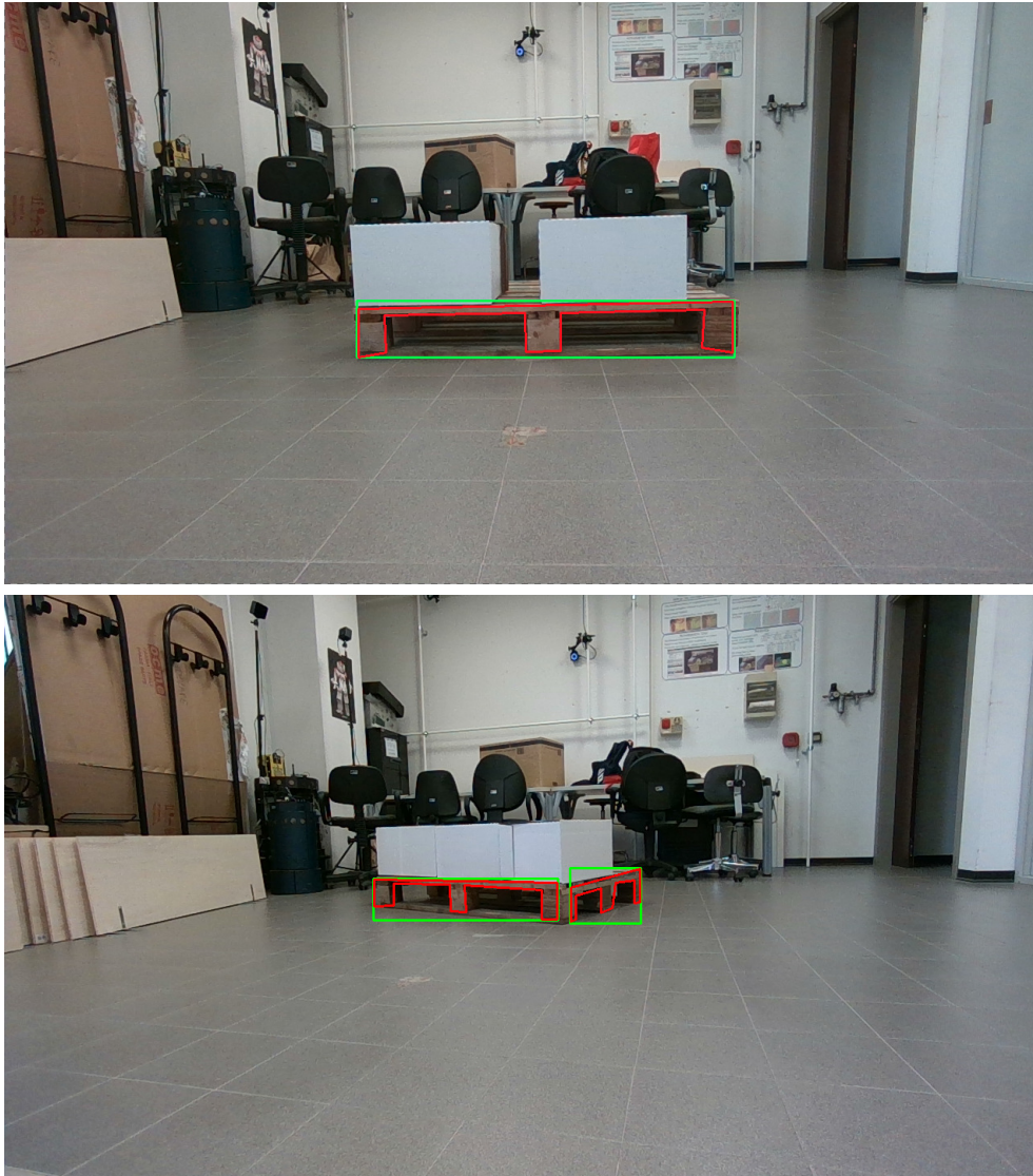
Figure 4.9: Examples of detections. The green rectangle is the bounding box. The red lines connect the keypoints.
