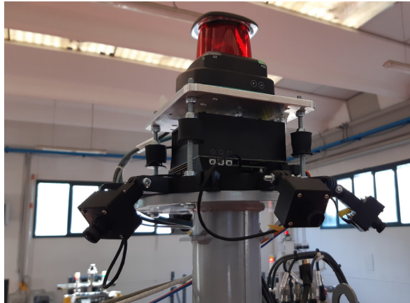
Figure 2.8: Onboard computer vision system on the AGV including a Jetson AGX Xavier board and multiple RGB cameras.
