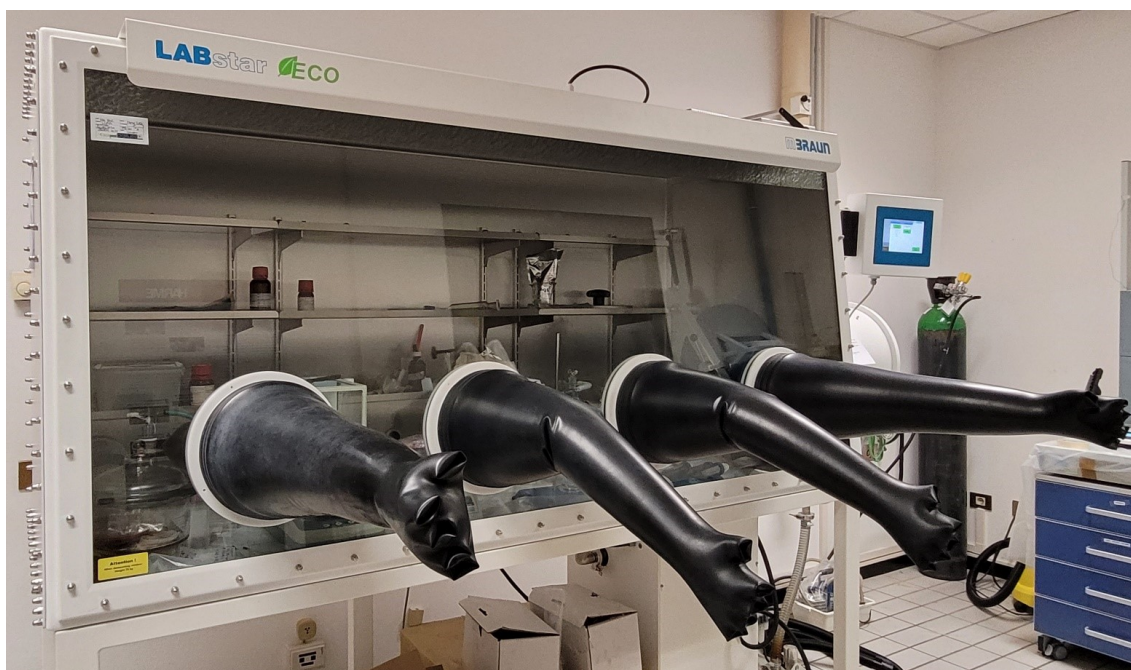
Figure 3.11. Glovebox (LabStar, MBraun, Germany) under Ar atmosphere used for infiltration with air and moisture sensitive preceramic precursor.
