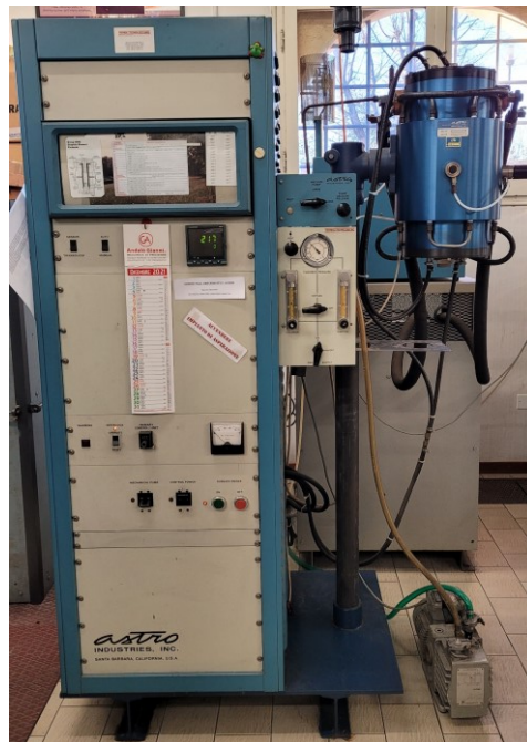
Figure 3.15. Resistance-heated graphite furnace (1000-3060-FP12, Astro Industries Inc.) used for pyrolysis cycles at temperature in the range 1100-1900 °C under Ar atmosphere.
