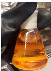
Figure 8.3. Polycarbosilane SMP-10 after heat treatment at 90 °C.
