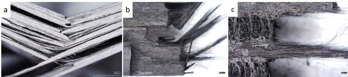
Figure 5.12. Optical images of a fractured bar reported as examples of fractures of (a) sample 0/0°, (b) sample 2D_tw and (c) sample 2.5D.
