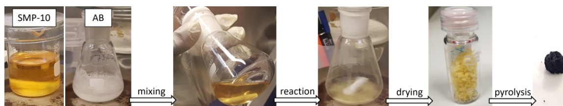
Figure 8.5. Scheme of the processing and resulting synthesis products until SiBCN(O) ceramic formed: 1) starting materials: pure SMP-10 and solution in THF containing ammonia borane (AB), 2) SMP-10 and AB solution after mixing (evolution of gases), 3) solution after heating under THF reflux for 30 min, 4) solid single-source precursor upon drying, 5) SiBCN(O) ceramic after pyrolysis at 800 °C for 12 h.
