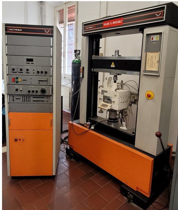
Figure 3.34. Screw-driven load frame (Instron mod. 1195, Instron, USA) equipped with a furnace (HTTF mod. 924, Severn Furnaces Limited, UK) for bending tests at high temperature.
