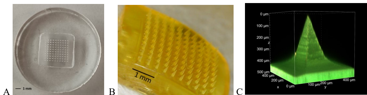
Figure 27: A) representative image of MPatch™ Microneedle Template ST-14, B) image of soluble microneedles array (obtained with Jiusion USB Digital Microscope) and C) two-photon microscopy visualization of a single microneedle (excitation wavelength 820 nm).
