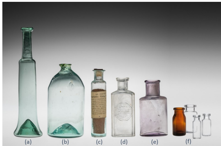
Figure 1.1 Evolution of pharmaceutical container shape, size, color, and glass composition from 1600s through today. From left to right: (a) manually free-blown soda-lime bottle circa 17 th century, (b) manually mold-blown soda-lime bottle circa 18 th century, (c) manually mold-blown soda-lime vial circa 1840–1860, (d) manually mold-blown soda-lime bottle circa 1865–1915, (e) semi-automatically mold blown soda-lime bottle circa 1880–1920, and (f) borosilicate vials: mold blown amber and tubular converted clear circa 2013–2016. Objects a–e are from the collection of the Corning Museum of Glass, Corning, NY [1].
