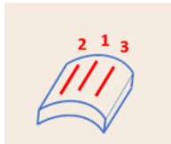
Figure 4.6 Schematic view of the 3 scratches applied on the same sample spaced approximately 3 mm apart, approximately.
