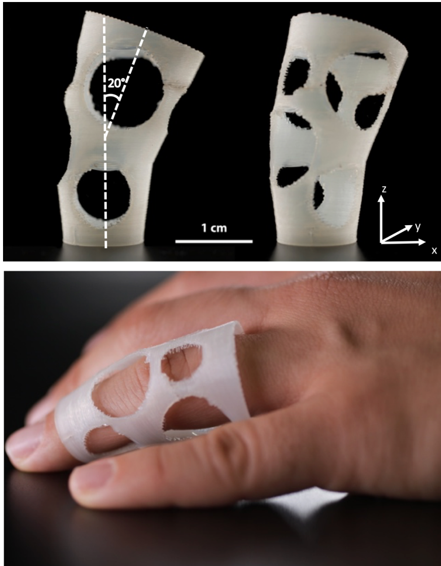
Figure 58 - Complex shaped object as a finger cast 3D printed by a filament of PHBH+CNC_AC_10, used as personalized medical device in case of finger dislocation.
