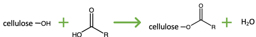
Figure 13 - Scheme reaction of esterification procedure.
