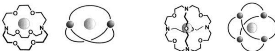
Fig. 5.22: Simplified scheme displaying the structural analogies between cryptands, interconnected crown ethers, and metallacryptands.
