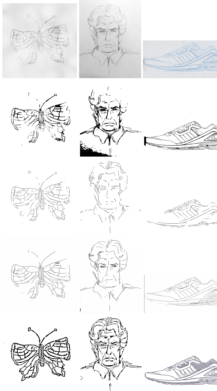
Figure 3.20: Comparisons for the line extraction step: an image from our inverse dataset - first column; a random sketch from the internet, author: Michael Bencik - second column; a real Adidas AG TM hand drawn design - third column. Results are obtained from: a commercial tool in second row, two state of the art algorithms ([2] in third row and [4] in fourth row), and our method in the bottom row.
