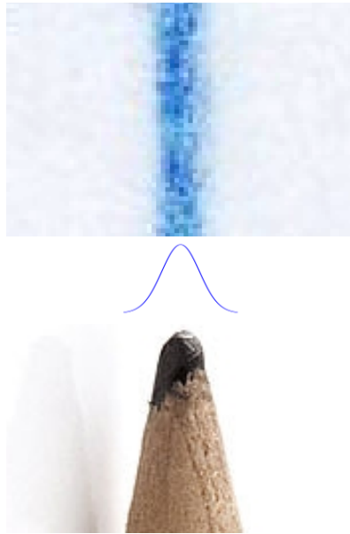
Figure 3.3: Perpendicular sections of a pencil line can be well approximated by a bell-like function (e.g. Gaussian or arc of circumference). The trait intensity has a strong correlation with the pencil tip that traced it.
