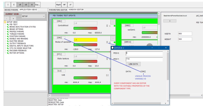
Figure 3.24: C.I.T view, component properties editor and mapped variables linking.
