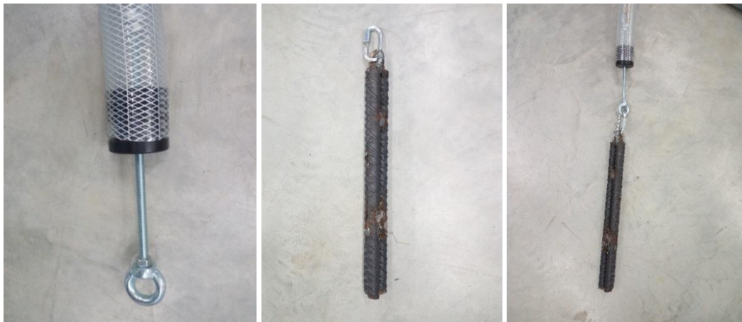
Fig. 3.21: Appearance of the chain-anchor connection system
