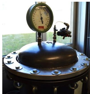
Fig. 3.10: Autoclave used for the calibration of piezometers
