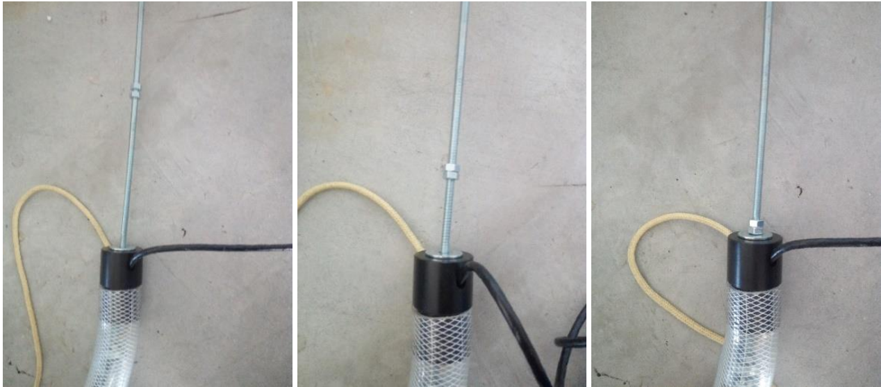
Fig. 3.23: Once Vertical Array is placed inside the borehole, it is necessary to screw the bolts along the bar until they reach the plug
