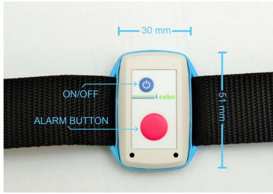
Fig. 2. MuSA wearable sensor.
