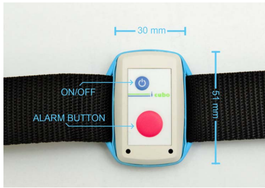
Fig. 2. MuSA wearable sensor.
