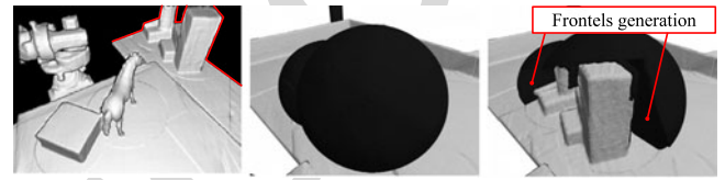
Fig. 9. Effect of the volume padding on frontel generation, during first NBV of scenario 2. Left: KinFu output, with the TSDF volume limit highlighted in red. Center and right: surfels/frontels before and after the NBV.
